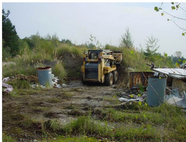
Fig. 1. Polluted site where the soil sample for laboratory experiments as well as for pilot-scale demonstration was taken (sampling by use of small loader).
